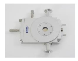
The THMS350V heating and freezing vacuum stage
