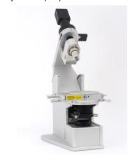
Linkam Imaging Station. Optics are tilted back to allow easy access to sample
