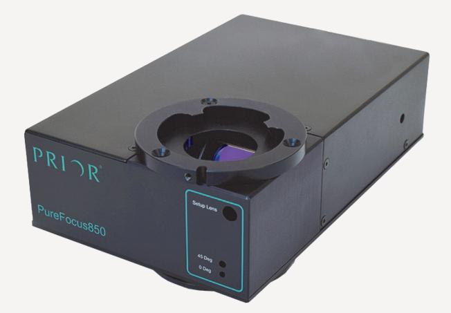
Prior Scientific's PureFocus850 combines advanced optics and intelligent in-built microprocessing to provide a real time focus system for infinity corrected optical systems. A motorized offset lens allows real-time adjustment of the imaging depth into the sample, continuously holding the precise distance between imaging focal point and a reference boundary of choice.
