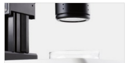
The working distance of 61.5mm leaves plenty of free room under the objective
