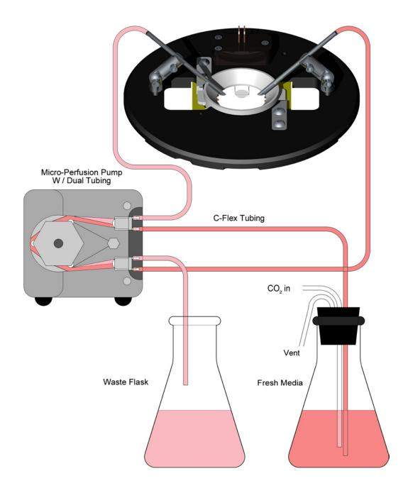
The Delta T Micro-Perfusion Pump is equipped with a dual tube manifold. The tube with a black ring on it has a slower fluid transfer rate than the other tube. The fresh media supply is coupled to this slow flow tube and the dish aspiration needle is attached to the faster flow tube. The level in the dish is controlled by adjusting the depth of the aspiration needle. This technique works well with all Delta T perfusable accessories.
