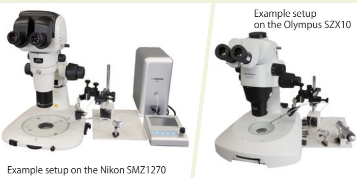
Example setup on the Nikon SMZ1270
