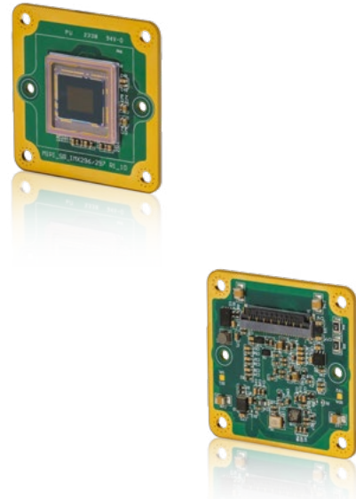
22-Pin Single-Board Camera Module
