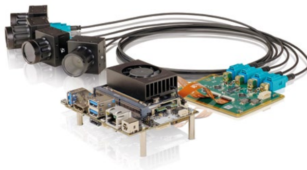
Reference Design: Carrier Board With NVIDIA Jetson Orin NX/ Nano SoM and up to four Acuva GMSL2 IP67 cameras
