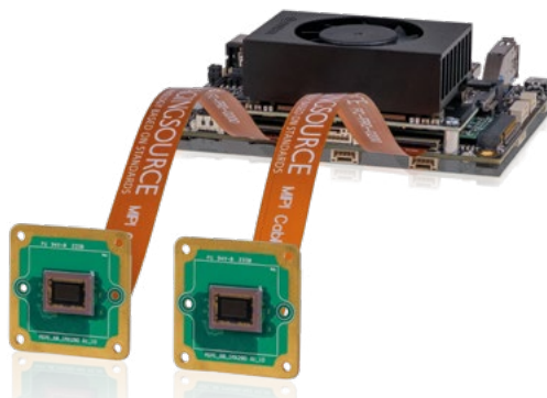
Reference Design: Carrier Board With NVIDIA Jetson Orin SoM and MIPI CSI-2 36S Cameras
